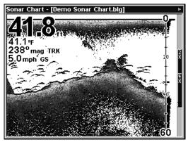
The overlay data on this sonar display includes, Depth, Temperature, Ground Speed and the Track the boat is following.
